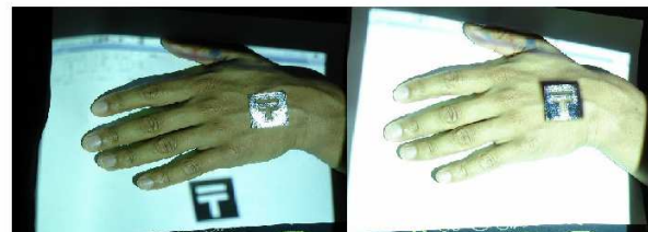
Fig. 7: Left: CG overlapping without calibration; Right: with calibration, the real marker and the projected one are overlapping.
