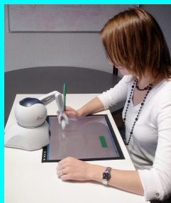
Subject undergoing the experiment “What You See Is What You Feel” interface. The force feedback device's stylus served as a pen over a simple flat screen, which served as a paper.
