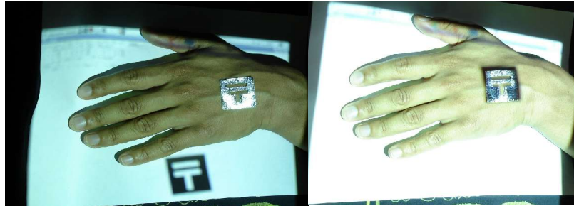
Fig. 21 - Calibration process. CG overlapping before calibration(left) and after calibration (right)
